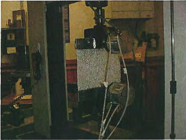
The preform tensile test determines the tensile load of a fiber glass preform or a glass mat. The specimen is cut to a 12"x 12" test size and is then clamped into test position with Pneumatic Grips using maximum air pressure. The test is run at a crosshead machine speed of 0.20 in/min. Once the specimen has reached maximum load the crosshead returns and the test is completed. The data recorded is Peak Load and Extension at Peak Load.
