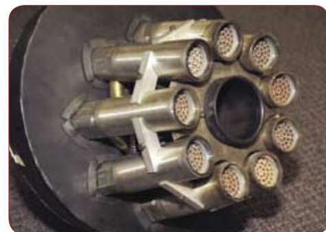
Electrically heated chopper head simultaneously dispenses and sets the string binder. The new system uses proportional control of fiber deposition based on tool velocity and modulated air flow during forming to control loft and reduce energy. The preform tooling, which determines the fit and shape to the mold, is also upgraded to reduce fiber distortion in the part.
