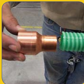
This $123 customized fitting and off the shelf hose saved nearly $650!
