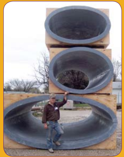
MFG CP teammate sending off the custom 19-foot elliptical shaped forms to NY. These forms produce columns for the Beekman Tower, a 75-story glass and titanium-skinned residential project in downtown Manhattan.
